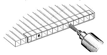
Extruded ribs shall be installed in a vertical direction for drainage.
